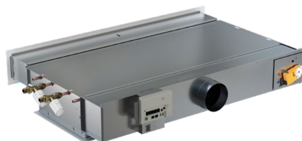
Figure 12. WISE Paragon with water connection on the left side. Complete product with factory-installed WISE CU control unit, actuators, and valves and valve actuators for cooling and heating water.
