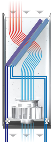
UDW: Downflow delivery, chilled water, dual circuit
