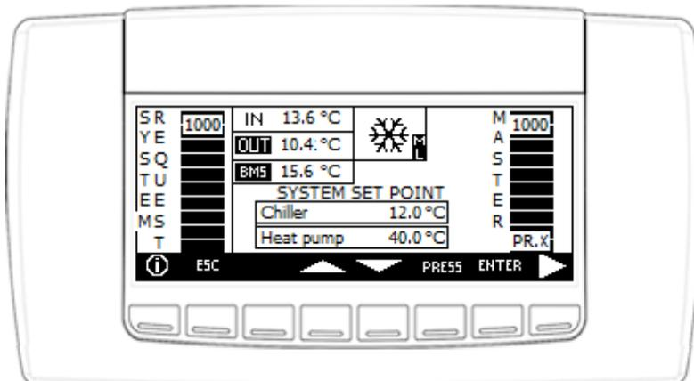
Fig. 13 Main screen of the Master regarding the Multilogic function
