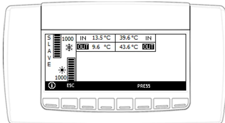
Fig. 54 Screen of the Slave units regarding the Multilogic function
