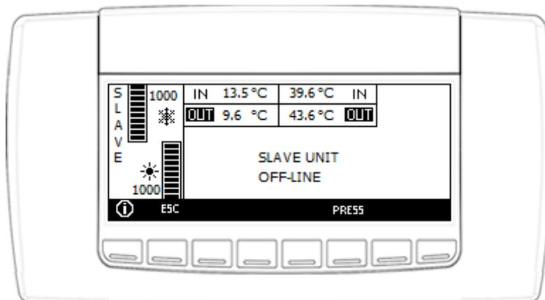
Fig. 55 Screen of offline Slave units relating to the Multilogic function
