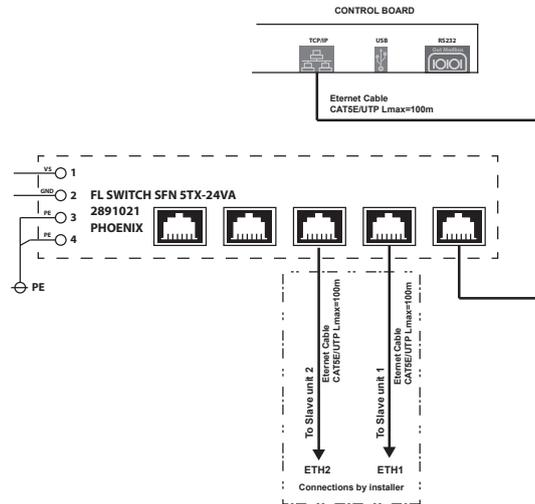
Fig. 59 Ethernet switch for Multilogic network in Master unit - example
