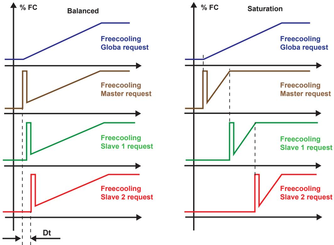
Fig. 20 Activation of fans in Balanced and Saturation mode
