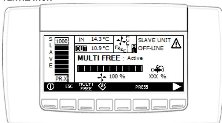
Fig. 38 Slave screen for standard version
