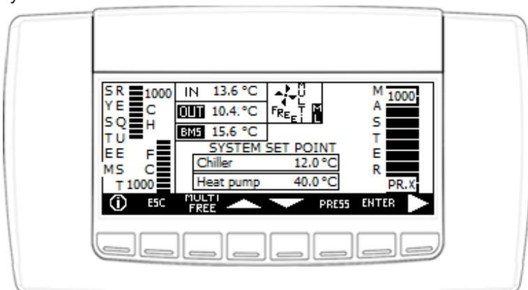
Fig. 28 Main screen of the Master regarding the Multilogic system with Multifree function active
