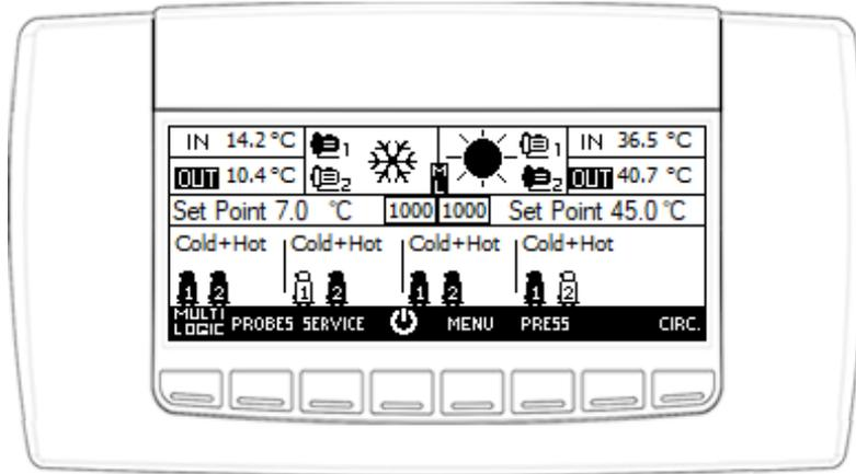
Fig. 51 Main screen of a multi-purpose unit regarding the Multilogic function
