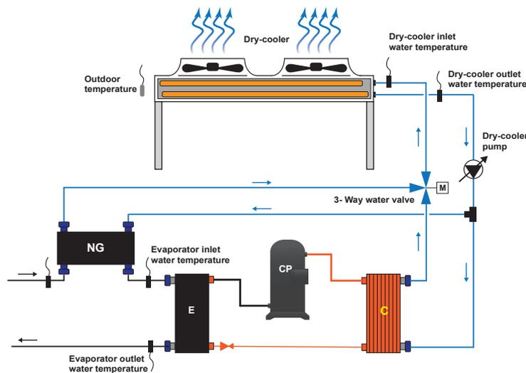
Fig. 23 Diagram illustrating a freecooling water/water, no glycol unit
