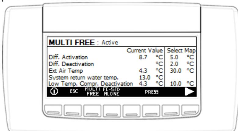
Fig. 43 Water/water units - General Master Multifree screen
