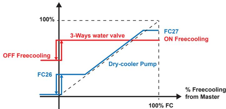
Fig. 25 Operating curves of 3-way water valve and dry cooler pump
