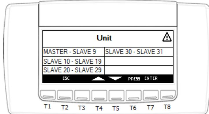
Fig. 29 Master Screen displaying all the units present in the installation
