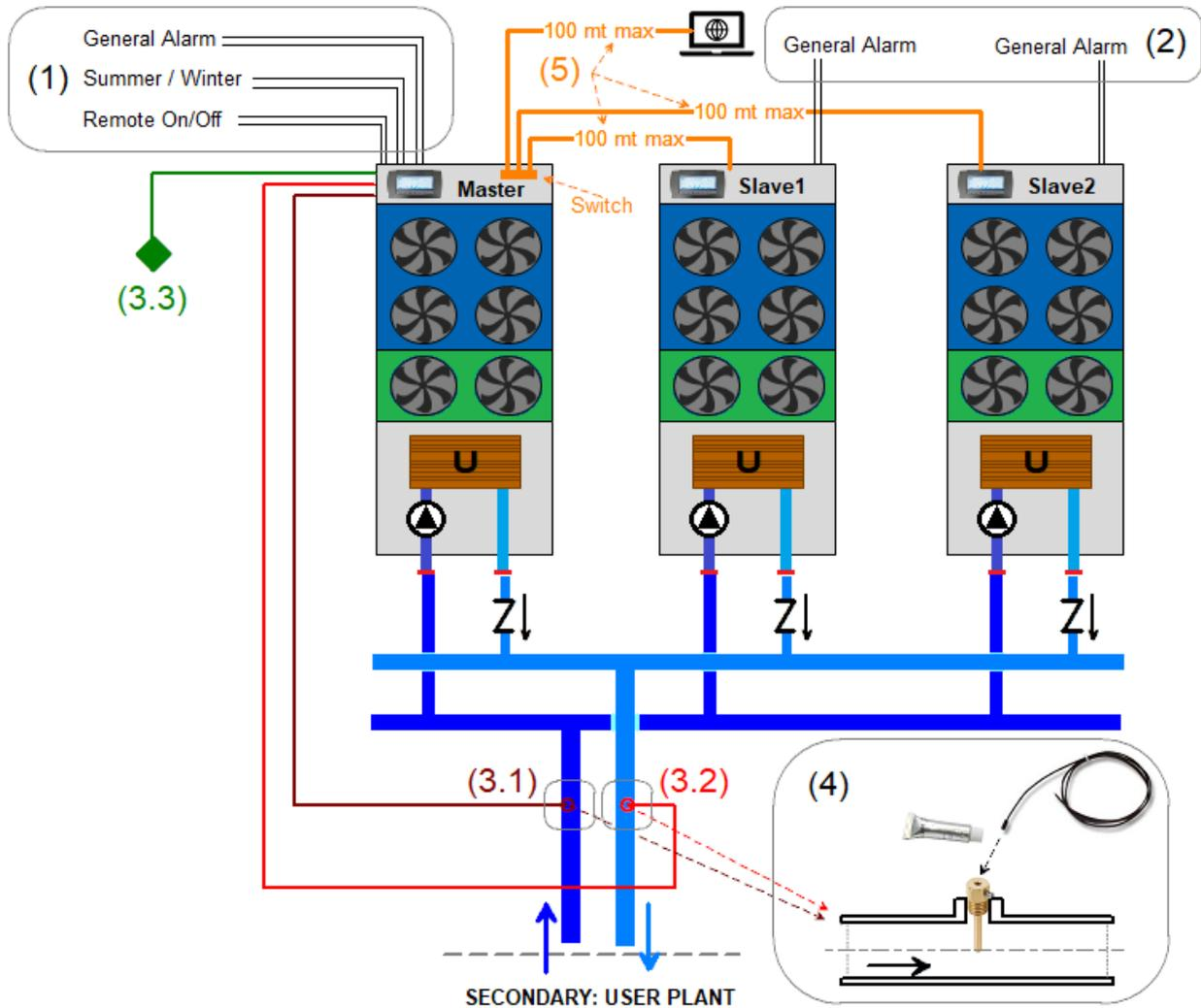
**Section (1):** optional basic connection to the Master unit (example for CH&CH-FC or CH&HP): for every supply must be checked the possible connections to the Master in according with the unit type. For example, if there are multi-purpose 4-pipes units, to the Master is possible to connect the remote ON/OFF for the hot and cold side as well.
