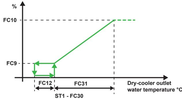
Fig. 24 Diagram illustrating how to set the speed of the dry cooler fans in freecooling mode
