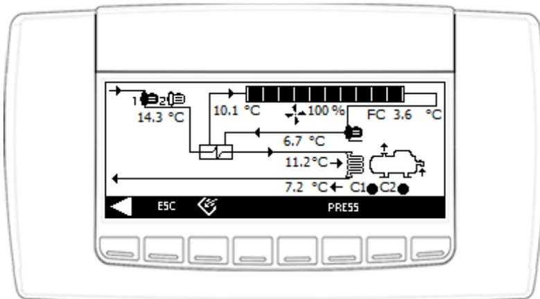
Fig. 42 Slave unit with screw compressors and in no glycol version
