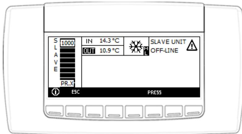
Fig. 17 Screen of the Slave units regarding the Multilogic function
