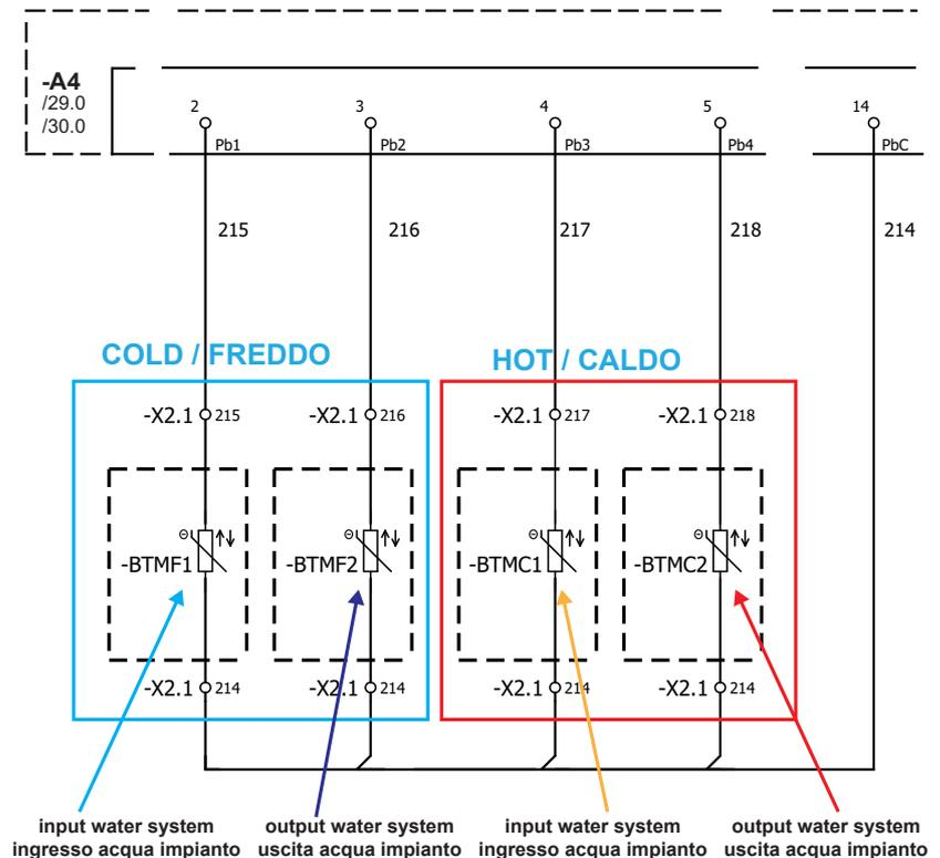
Fig. 57 Multilogic probes on Master with multi-purpose units
