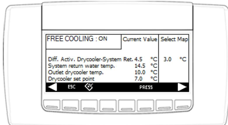
Fig. 46 Water/water units - Specific Master Multifree screen
