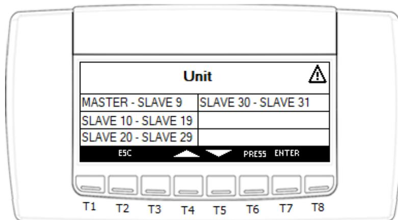
Fig. 14 Master Screen displaying all the units present in the installation
