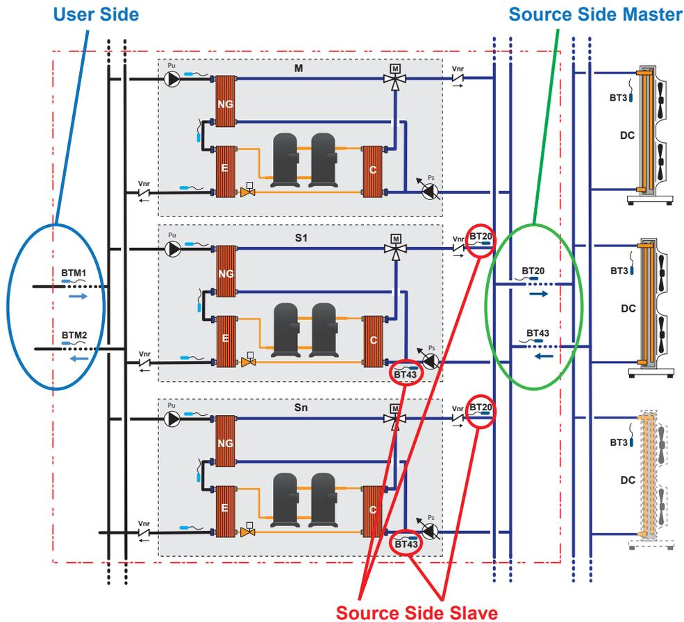
Fig. 58 Position of system probes: example of Multilogic / Multifree system, water/water, no glycol
