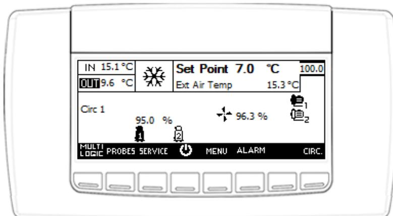
Fig. 12 Main controller screen
