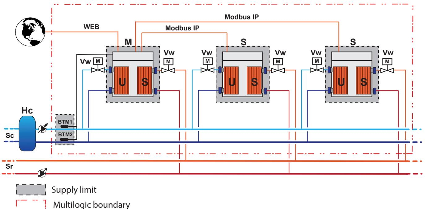
Fig. 11 CH water/water unit
