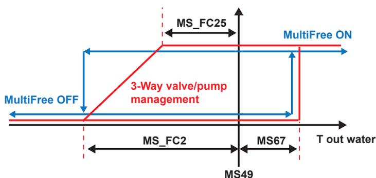
Fig. 19 Freecooling valve/pump control in air/water units
