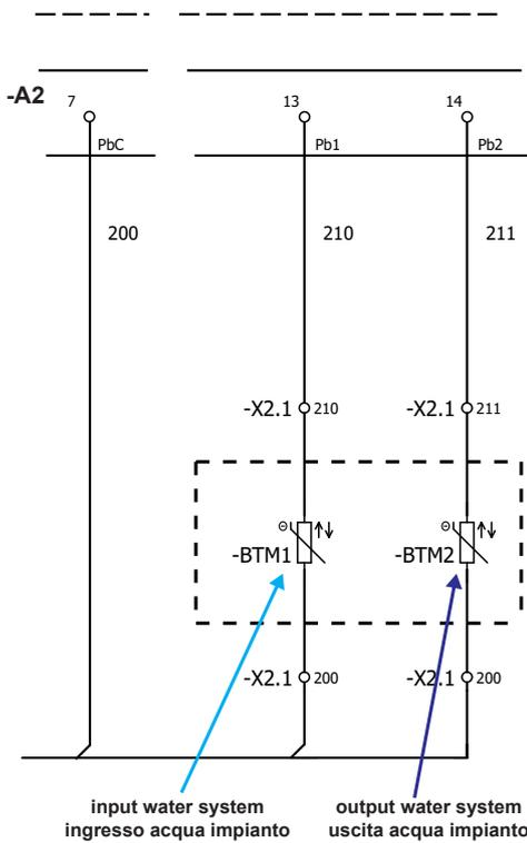
Fig. 56 Multilogic probes on CH or HP, air/water Master unit
