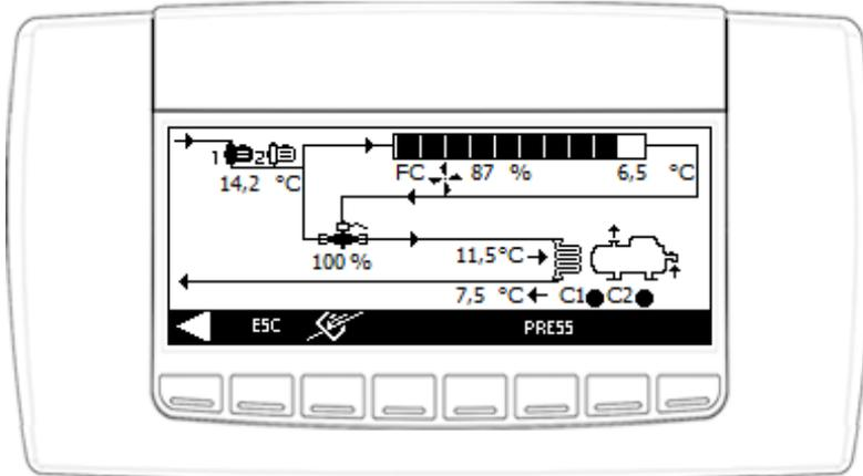
Fig. 41 Slave unit with screw compressors and in standard version
