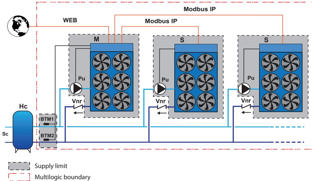
Fig. 8 CH air/water unit
