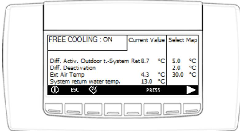
Fig. 45 Water/water units - General Master freecooling screen
