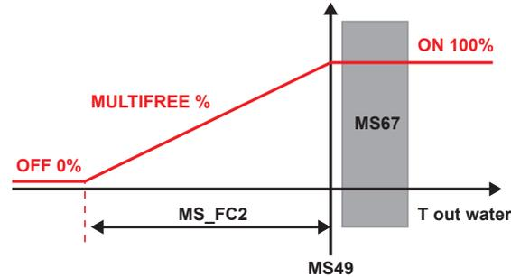
Fig. 22 Multifree freecooling percentage with water/water no glyco units
