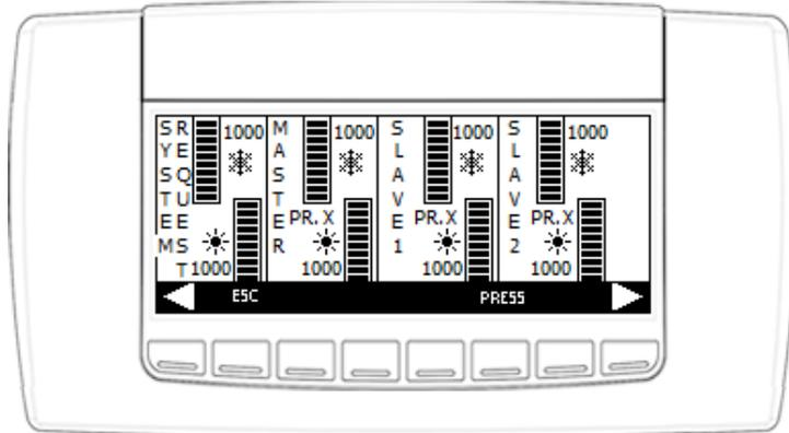
Fig. 53 Main Master screen with capacity distribution
