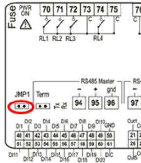
Fig. 3 Position of jumper JMP1
