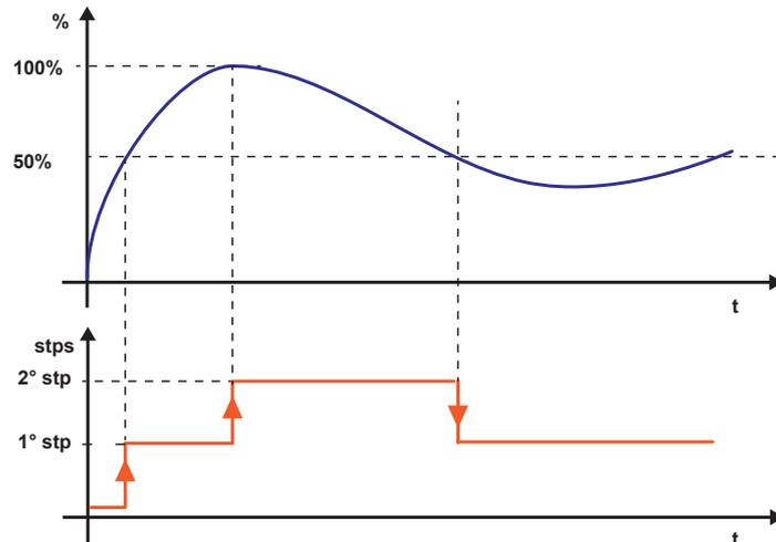
Fig. 21 Transformation of freecooling ventilation demand into two steps
