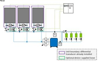
All system units must include the option "Variable flow unit arrangement for HYZER X"
