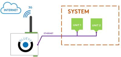
**Blueye**® is a supervision platform for remote monitoring of the HYZER X system using a network featuring a Modbus protocol.
