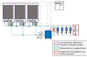
All system units must include the option "VPS and VFPP setup for HYZER X".
