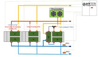
The acronyms in the HTC1 and HTC2 diagrams refer to the temperature probes supplied with the unit (2 in each user-side circuit - installation and wiring by the customer).
