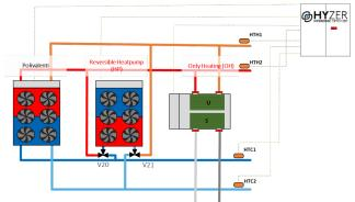
The acronyms in the HTC1, HTC2, HTH1 and HTH2 diagrams refer to the temperature probes supplied with the unit (2 in each user-side circuit - installation and wiring by the customer).
