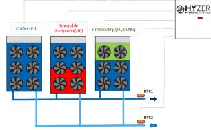
The acronyms in the HTC1 and HTC2 diagrams refer to the temperature probes supplied with the unit (2 in each user-side circuit - installation and wiring by the customer).
