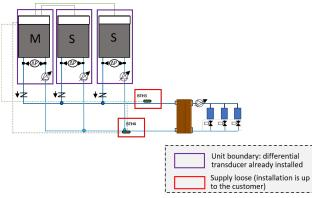
The HYZER E VPS with TD-based control function combines the Multilogic function, which is used to manage multi-machine systems, with the FLOWZER VPS with DT-based control control for variable flow systems.
