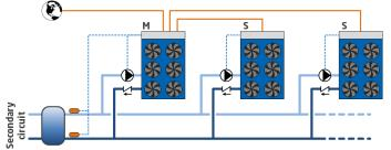
On the basis of the information recorded by the temperature probes installed on the delivery and return manifolds of the system, with the master unit, a capacity request is generated that is distributed among the units connected in the Multilogic network according to settable priority and optimization logics.
