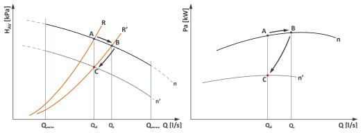
The use of the Flowzer allows the pump speed to be set manually (e.g. at speed n' instead of n) to obtain the design water flow rate and thermal gradient (point C). Once the adjustment procedure has been carried out, the pump will always work at a fixed flow rate.
