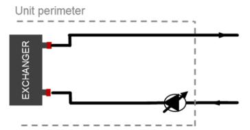
The accessory consists of inserting an inverter in the machine to manually adjust the speed of the pump (or pumps) in order to calibrate the pump flow rate on the head losses of the system.
