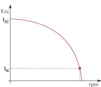
For an individual compressor, the normal starting current ISC will be 4-5 times its rated current IN.
