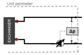
Flowzer VD requires two pressure transducers to be installed in the machine. Through these transducers, the inverter can gauge the actual pressure at the ends of the system and it can automatically adapt the pump speed to obtain a set available discharge head value. Flowzer VD must be combined with Flowzer VP. This accessory therefore allows a constant pressure system to be achieved.
