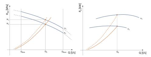
Flowzer VDE is used to automatically adjust the pump speed. As the graph shows, the inverter trips and increases the pump speed if a different condition occurs which would cause an undesired drop in the flow rate (e.g. operation of an external dry cooler). This is a more accurate solution than the VP option alone as it always provides for the water flow (Qd) required by the design conditions.
