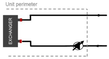
The accessory consists of inserting an inverter in the machine to manually adjust the speed of the pump (or pumps) in order to calibrate the pump flow rate on the head losses of the system.
