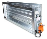
The GLOBAL LPFW units can be equipped with motorised dampers delivered pre-wired to cut draughts when the unit is deactivated. They are delivered with a pre-wired servomotor and are controlled entirely by the regulation system. A starting delay of the fans is designed to allow the damper to open first.
