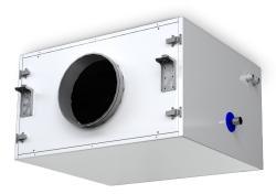
The external insulated casings are fabricated in galvanized steel sheet. the outer sheet is painted in RAL9002. The double-skin panels contain 30mm mineral wool. ..The casings can be use to integrate external cooling, heating, direct expansion coils (EBA) .
