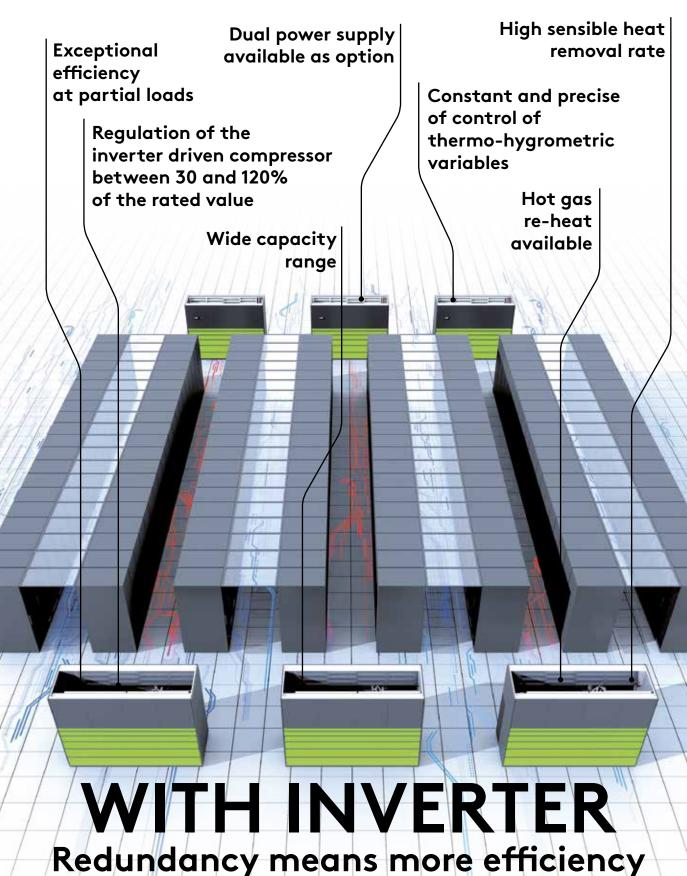
The higher efficiency of the refrigerant circuit at part load conditions grants the maximum benefit in (n+1) redundancy applications
