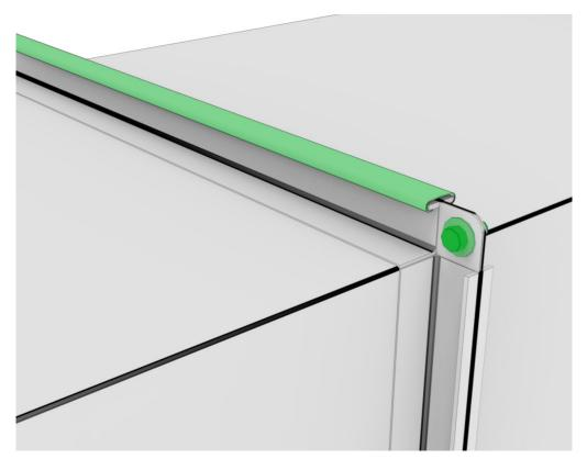
Figure 4. Installation of Euroflange
