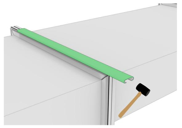
Figure 2. Installing the guide rail
