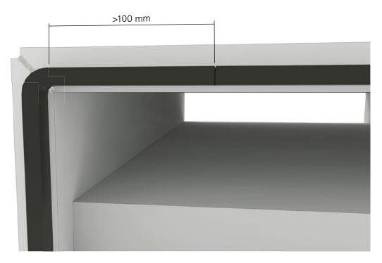
Figure 1. Slip-clamp with gasket
