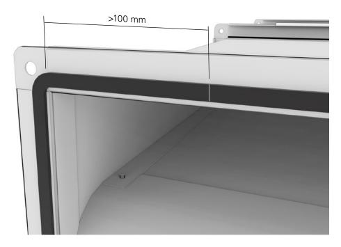
Figure 3. Euroflange with gasket
