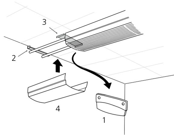
Figure 4. Cover for connection against a wall.
