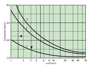
Curve 1 Plenum/Duct; Curve 2: Duct/Plenum, Curve 3: Plenum/Plenum
