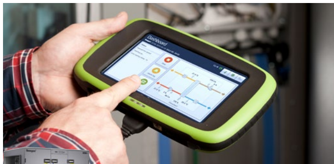
GOLD is controlled via a user-friendly touch screen, but can also be controlled via mobile phone, computer or central building automation.
