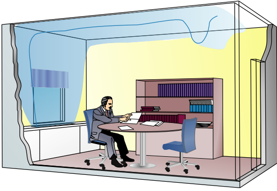
Figure 43. Perimeter wall units installed below windows in a cellular office.
