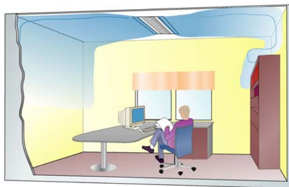
Figure 36. Corridor–perimeter wall-oriented climate beams in cellular offices.
