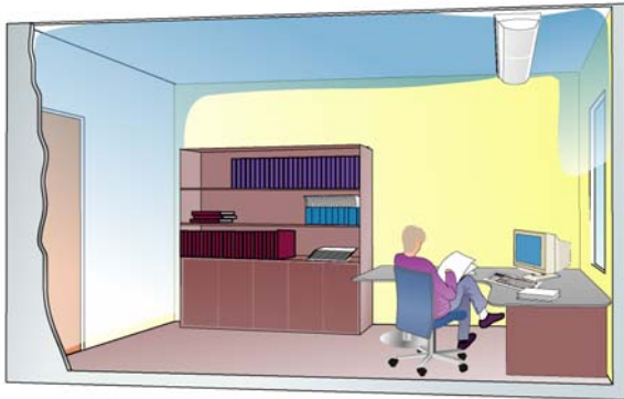
Figure 38. Climate beams installed at the front edge in cellular offices.
