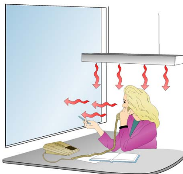
Figure 4. Radiant transfer occurs between all surfaces that have different temperatures irrespective of the direction.
