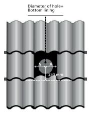
1. Mark out where the hood will be placed. Affected tiles are removed. Make sure that you do not end up above a roof truss, or other inappropriate place. Drill the hole perpendicularly to the ceiling. In height, the centre of the hole should be 230 mm from the bottom of the tiles. Sideways, the hole is placed in the middle, measure A to be equal. When mounting Ø200 and Ø250 the distance is 400 mm from the bottom of the tiles to the centre of the hole.
