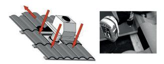
3. The above-lying tiles is pushed up against the ridge to facilitate mounting of the top lining. Assemble the top lining at the same angle as the roof. This is done by placing the isolated duct through the bottom lining. Then screw the top lining in the existing battens.
