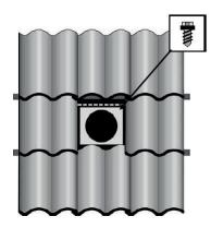
Make a cut in the roof felt, and insert 20 mm of the bottom lining under the felt. Fasten with the supplied screw. Seal the joints and screws with water resistant sealing compound
