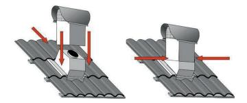
4. Install the top vertical, screw it to the top lining with the supplied screws. After the assembly the overlying tiles are pushed back to its original position.
