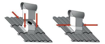
4. Install the top vertical, screw it to the top lining with the supplied screws. After the assembly the overlying tiles are pushed back to its original position.
