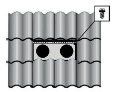
2. Make a cut in the roof felt, and insert 20 mm of the bottom lining under the felt. Fasten with the supplied screw. Seal the joints and screws with water resistant sealing compound.
