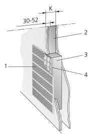
Figure 4. Flush mounting measurements for the DIR.
