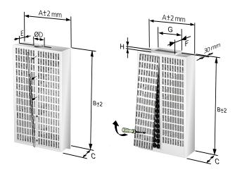
Figure 7. Maintenance for two-piece front with A=1190 mm and circular connection, dismantle the cover strip and then the screws that secure the front plate, lift and pull out.
