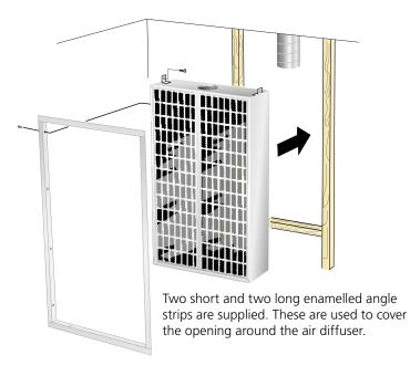
Figure 3. Recessed installation.
