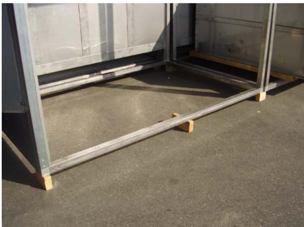
No foreign components / small parts should be stored in or on the assembly components. Movable components, such as the ventilator, rotary heat exchanger, doors, etc., should be secured against unintentional movement. Assembly components may not be stored in the danger areas from other machines.
