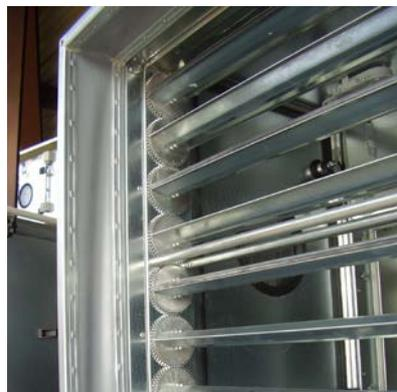
The louver damper positioner can be mounted on the interior, as well as on the exterior of the housing. It should be mounted on the interior of those units designed for outside use, or protected against moisture.
