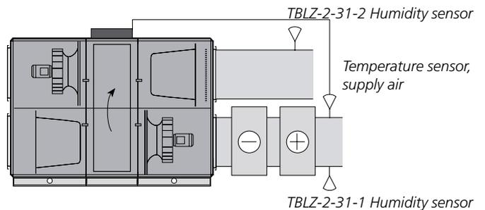
The TBLZ-2-31-1/2 humidity sensor should be mounted in the supply air duct and its cable should be connected to the appropriate terminal on the air handling unit.
